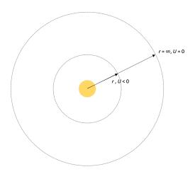
Visualizing how potential energy changes at varying "r" from a center point. Infinitely far away it has zero potential E and it loses potential E as it goes closer to the center, so the potential has a negative value. Diagram credit to <u>crashwhite.com</u> and analysis of diagram inspired by <u>crashwhite.com</u>'s description of the diagram.
