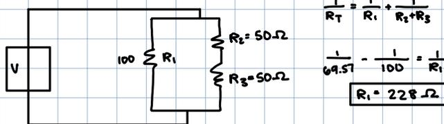
$$\frac{1}{R_T} = \frac{1}{R_1} + \frac{1}{R_2 + R_3}$$
