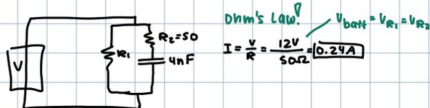
Ohm's Law!  $V_{\text{batt}} = V_{R_1} = V_{R_2}$
