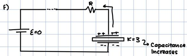
the charge left on these plates during discharge is  $Q = CV_0 (e^{-t/RC})$  greater than the charge during charging at  $t = 4s$ . Since there is a dielectric, the capacitance has increased, so the max  $Q$  has increased.
