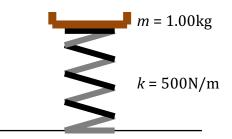
A spring of negligible mass and spring constant 500 N/m is oriented vertically as shown. A flat 1.00 kg platform is then attached to the top of the spring.
