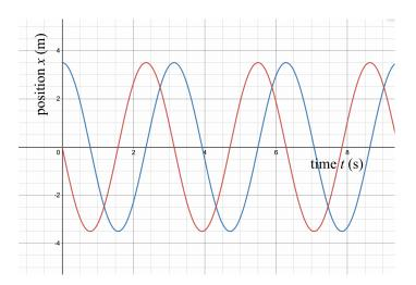
The same oscillator is set into motion, with time t = 0 when the mass is moving downwards and at the equilibrium position, as shown by the red line here.
