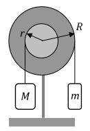
The pulley system consists of two solid disks of different radii fastened together coaxially, with two different masses connected to the pulleys as shown above. Under what condition will this pulley system be in static equilibrium?
