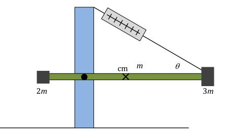
A weight of mass 2m is now firmly attached to the left end of the beam, and a mass of 3m attached to the right end of the beam.
