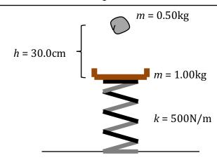
Now the platform is placed again at its equilibrium position. A 500 gram blob of clay is released from a height of 30.0 centimeters above the platform so that it falls and contacts the platform in a perfectly inelastic collision.
