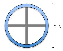
A pair of long, thin, rods, each of length L and mass M, are connected to a hoop of mass M and radius L/2 to form a 4-spoked wheel as shown above. Express all answers in terms of the given variables and fundamental constants.
