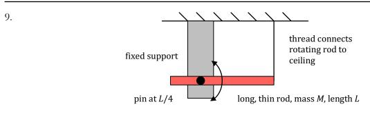
A long, thin, rod of mass M = 0.500kg and length L = 1.00 m is free to pivot about a fixed pin located at L/4. The rod is held in a horizontal position as shown above by a thread attached to the far right end.
