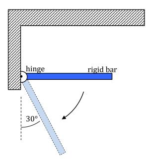
A rigid bar with a mass M and length L is free to rotate about a frictionless hinge at a wall. The bar has a moment of inertia  $I = 1/3 ML^2$  about the hinge, and is released from rest when it is in a horizontal position as shown. What is the instantaneous angular acceleration when the bar has swung down so that it makes an angle of 30° to the vertical?
