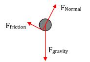
Note that the Normal force should originate from the point where the cylinder touches the surface, as should the force of Friction acting parallel to the plane. The force of gravity should originate at the center of mass of the cylinder.
