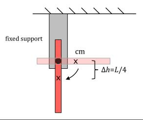
$U_{i} + K_{i} = U_{f} + K_{f}$   $mgh + 0 = 0 + \frac{1}{2}I\omega^{2}$   $mg\left(\frac{L}{4}\right) = \frac{1}{2}\left(\frac{7}{48}ML^{2}\right)\omega^{2}$   $\omega = \sqrt{\frac{24g}{7L}} = 5.80rad/s$
