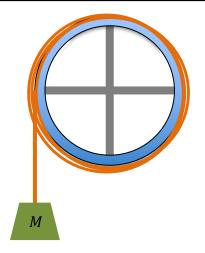
The wheel is now mounted to a frictionless fixed axle and suspended from a vertical support. Several turns of light cord are wrapped around the wheel, and a mass M is attached to the end of the cord and allowed to hang. The mass is released from rest.
