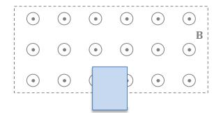
Now a rectangular conducting loop of width w and height h is dropped so that it has an initial velocity v as the lower edge of the loop enters the magnetic field at time t = 0. The loop has a mass m and a total resistance R.
