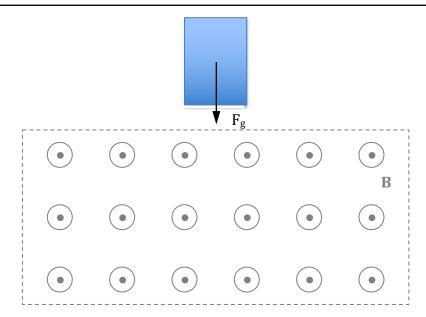
3. A constant horizontal magnetic field is directed out of the page as shown here. A thin, solid, rectangle of conducting material is held above the upper edge field and released so that it falls due to gravity.
