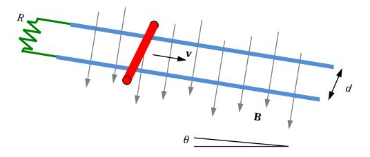
The entire apparatus—rails and magnetic field—is placed on a platform that allows the device to be tilted so that the rails are oriented at an angle  $\theta$  above the horizontal. The magnetic field **B** remains perpendicular to the plane of the rails.
