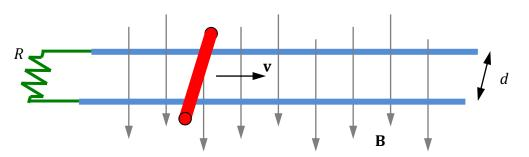
A load resistance R is now connected to the conducting rails as shown, forming a complete circuit with the sliding bar.
