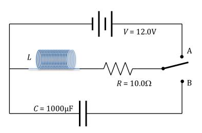
The solenoid/inductor is now placed into the circuit shown above, with the 12.0-Volt battery, the 10.0  $\Omega$  resistor, a switch, and an uncharged 1000 $\mu$ F capacitor as shown. The switch is initially open, and then moved to position A at time t = 0.
