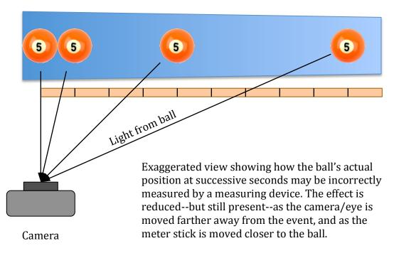
With a little work, you may be able to discover a formula that will allow you to determine the true location of the ball, based on the (incorrectly) measured location, the location of the meter stick, and the location of the camera. This would allow you to calculate the correct location of the ball.
