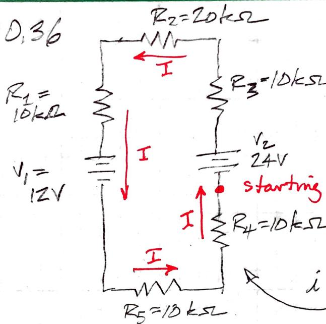
a) Find voltage across each resistor. To do this, we need to find current, which is relatively easy, given that there's just one loop & no junctions.
